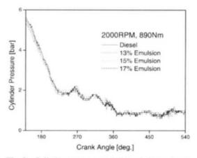
Fig. 8 Cylinder pressure variation during exhaust process
