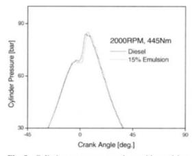
Fig. 5 Cylinder pressure comparison with emulsion fuel
