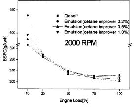
Fig. 10 Comparison of BSFC at 2000 rpm
