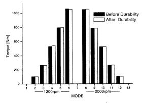
Fig. 12 Comparison of torque before/after durability test
