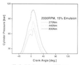
Fig. 7 Cylinder pressure at 2000 rpm
