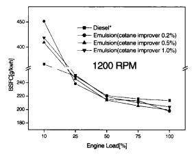
Fig. 9 Comparison of BSFC at 1200 rpm
