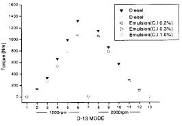
Fig. 4 Comparison of torques for various fuels
